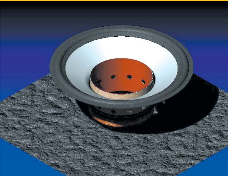
Figure 2. The computational model of the moving assembly of a loudspeaker: voice coil, voice-coil former, cone and surround. The model is used to calculate the resonant modes of the system for different cone materials.
